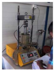
California Bearing Ratio test being conducted to measure the strength of the subgrade of a road
