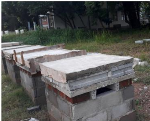
Small-scale physical models with insulation and the schematic view
