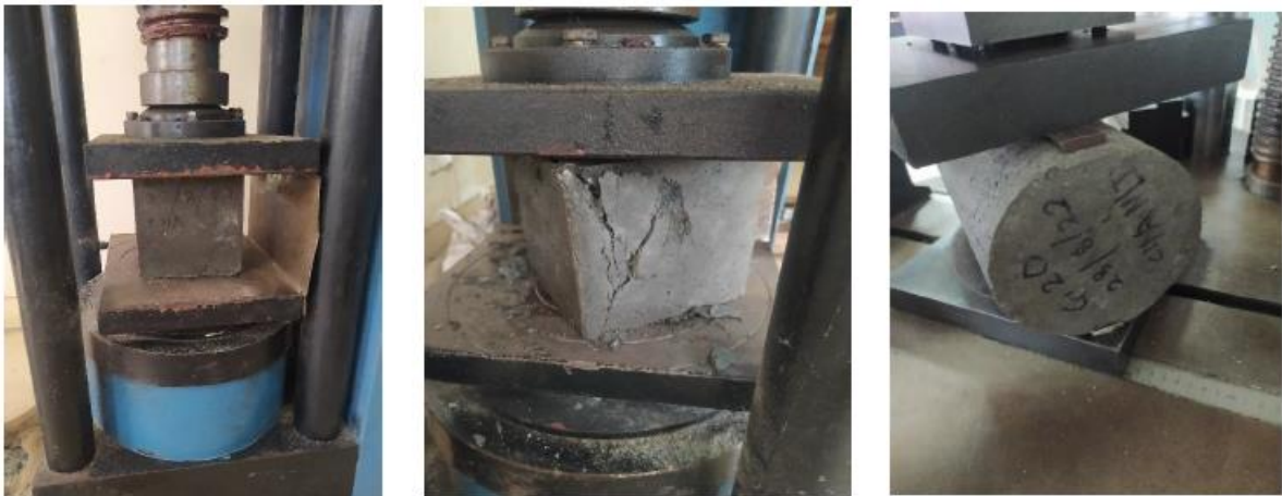
Coconut fiber added cube strength and cylinder splitting strength tests being conducted at lab
