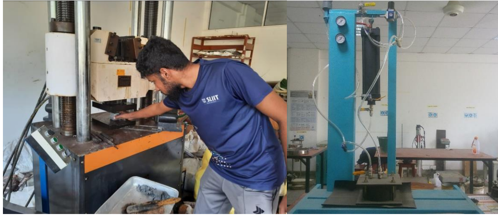
Testing of mechanical characteristics and permeability of modified material
