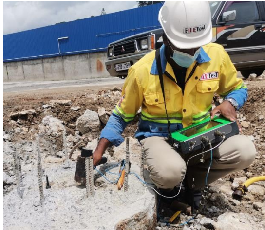
Carrying out the PIT using transient dynamic response method using an instrumented hammer
